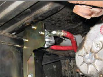
Using the filter mounting bracket or a cutout/trace as a guide, mark the 2 spots for the mounting bolts. The bracket will be positioned so that the filter will be pointing downward when installed (see picture to the left).
