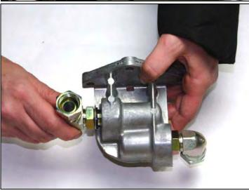
Install the two 90° ORB fittings (1604046) into the filter head (do not use pipe sealant). When installed, the fittings need to point toward the front of the vehicle. For ease of installation, we recommend assembling the fittings on the filter head on a work bench before installing it onto the vehicle.
