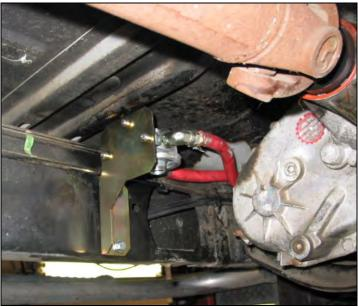
Position the filter mounting bracket and install the 2 mounting bolts using the flat washers supplied. Then, secure it using nuts and lock washers.
