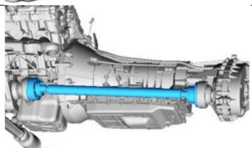
33. Install the rear driveshaft CV joint-to-transfer case flange cup bolts and retaining straps.
