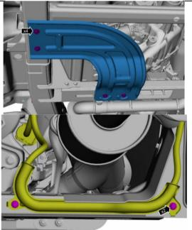
24. If equipped, remove both the LH and RH exhaust heat shield bolts from transmission crossmember.
