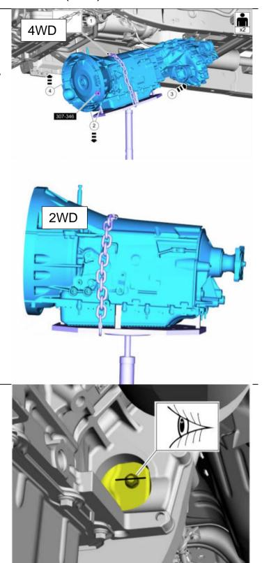
7. Install x3 top bellhousing bolts. Install x3 LH bellhousing bolts. Install x3 RH bellhousing bolt.
