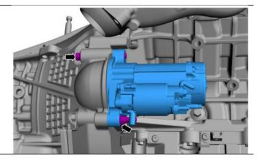
41. (1) Install the starter motor ground cable and secure with nut.
