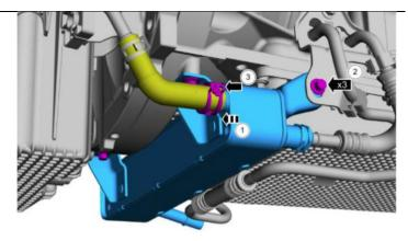
38. Connect the coolant hose to the transmission fluid cooler.
