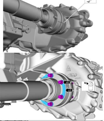
16. Remove the front driveshaft.
