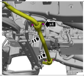
37. Install the transmission fluid cooler with the bolts and the hose clamp.
