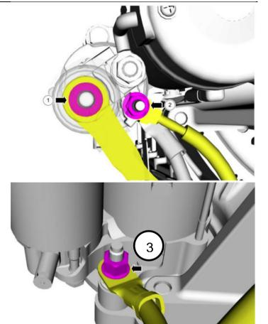
3. Remove the starter motor's three bolts and remove starter.
