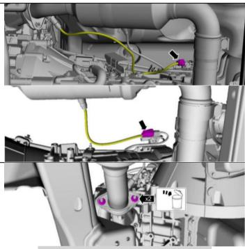
22. Remove the LH catalytic converter nut, then loosen the clamp to remove the catalytic converter.
