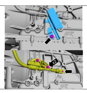
31. Remove fuel line bracket bolt.
