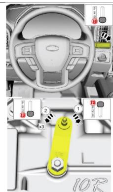
45. Connect the selector lever cable to the manual control lever, and lock it on.
