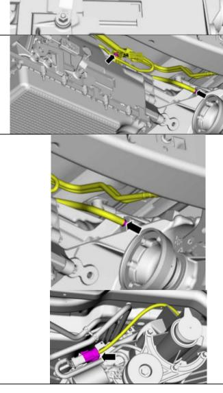
14. Install the selector lever cable bolts but keep the cable disconnected to the manual control lever.
