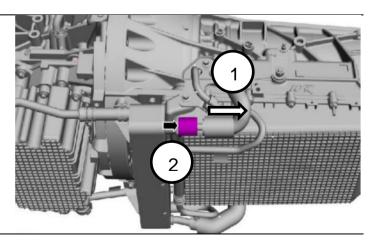
5. With the special tool (307-569), disconnect the transmission fluid cooler inlet tube from the cooler.
