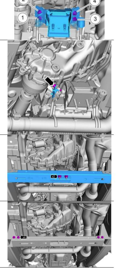
21. Install both LH and RH exhaust heat shield.
