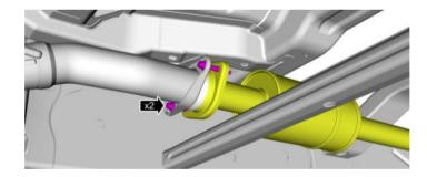
30. **If equipped**, remove splash shield by removing one bolt.
