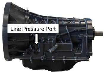
The line pressure service port plug thread is M10x1.00NPT.
