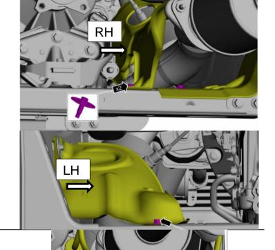
22. If equipped, install the wiring harness onto transmission crossmember.
