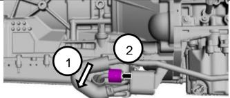
7. With the special tool (307-569), disconnect the transmission cooler outlet tube.
