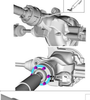
15. Index-mark the front driveshaft flange CV join-to-transfer case flange cup and then remove bolts and retaining straps.
