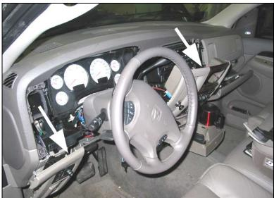
Measure and mark a spot for the toggle switch 3/4" up from the bottom edge of the dash panel and 1" in from the left edge of the accessory panel as shown in the photo.
