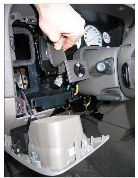
Once the switch is installed, attach the ground wire to a good metal ground under the dash.
