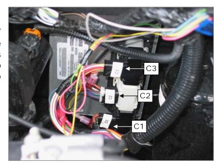
On connector C1, locate pin 23 (The orange wire/dark blue tracer and install a gray Posi-Tap to this wire. Plug the yellow DFIV wire onto the Posi-Tap.
