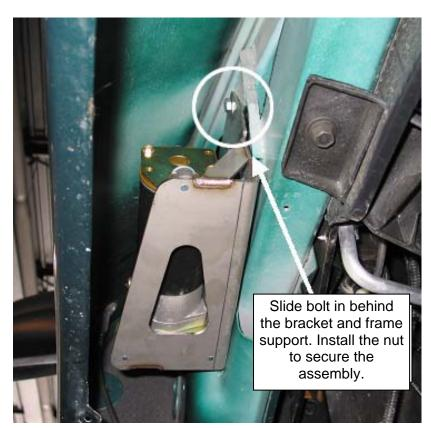
Tighten bolts all and secure assembly. Route the compressor pigtail wiring harness up towards regulator assembly the previously installed. You will also need to route a small section of plastic air hose from the quick connect fitting of the air compressor to the regulator assembly. Use the wiring diagram on page 15-16 as a reference for the wiring of the air hoses and the electrical wiring. NOTE: Be sure to keep all hoses and wiring harnesses away from any moving parts or heat sources.
