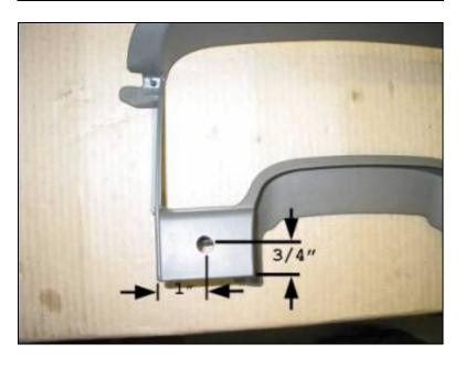
Install the switch into the newly drilled hole and secure it with a lock ring, then re-install the dash trim panels by reversing the removal procedure.
