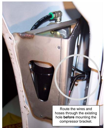
The wires and hoses must be fed up through the existing hole before tightening the compressor into place. Once this is done, re-install the hood support bolt. Raise the compressor assembly so that you can install the provided bolt through the frame hole onto the nut.
