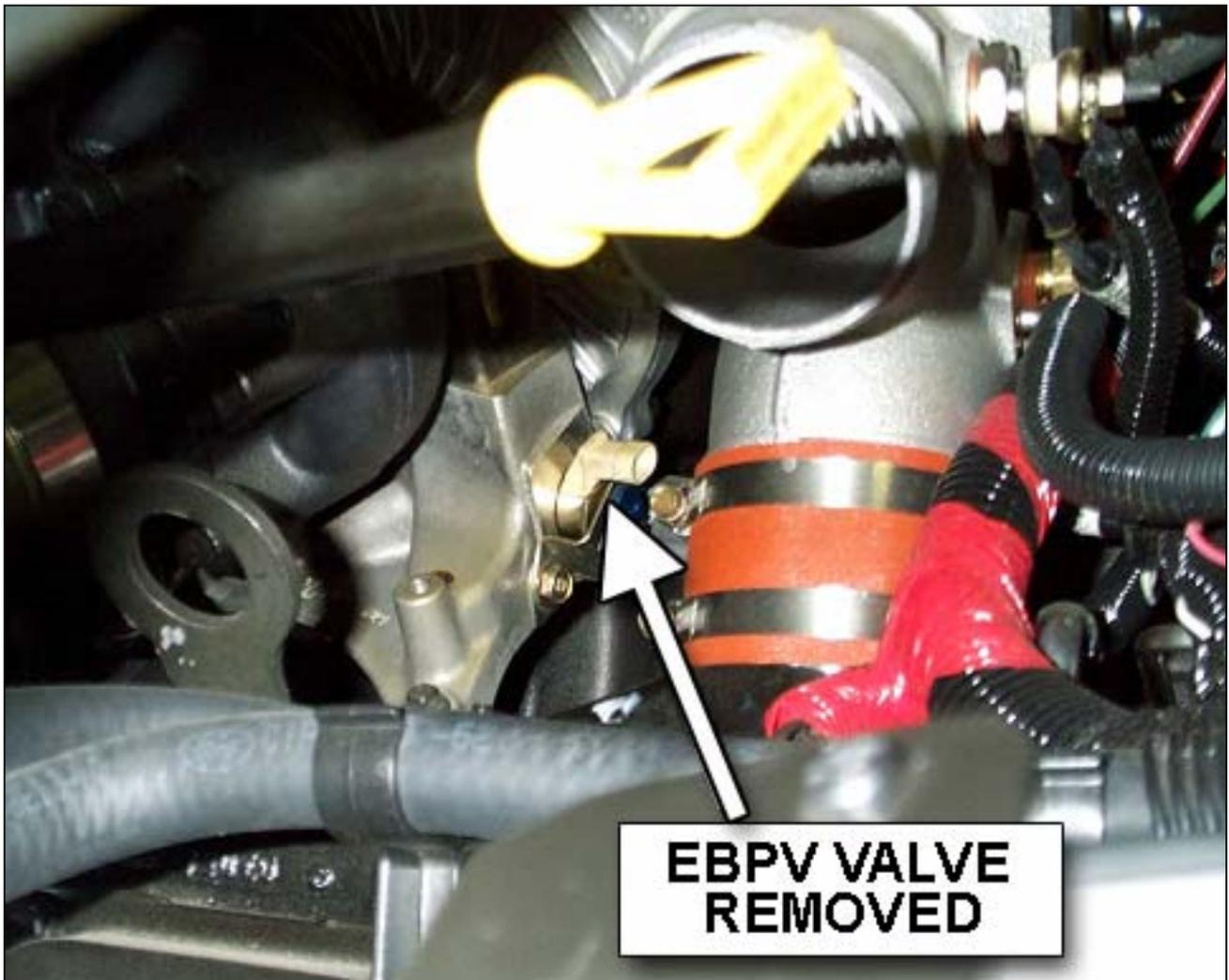
**NOTE: ON CALIFORNIA MODEL VEHICLES THE EBP VALVE WIRING MUST BE CONNECTED TO ENSURE THE ECM DOES NOT SET AN ENGINE TROUBLE CODE.**
