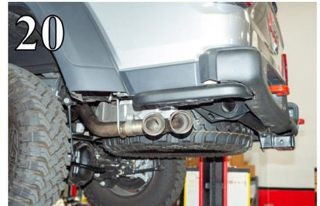
18. For Dual Side Cat-Backs, slide a clamp over the inlet of the tailpipe assembly (fig. 19) and connect it to the outlet of the over-axle pipe assembly (fig. 20).
