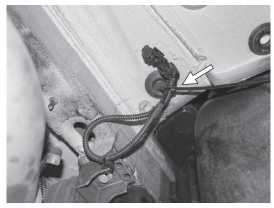
9) If installing a valveless exhaust system on a car with exhaust valves, install the two supplied dummy plugs onto the harnesses for the two flap motors. Use the supplied cable ties to secure the harnesses out of the way. Once complete, skip to step 17 of this manual.
