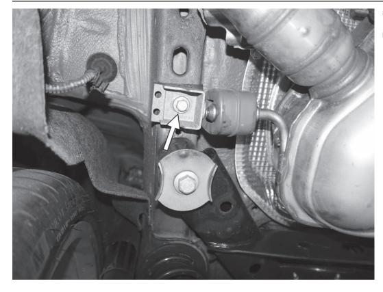
5) Loosen but do not remove the two 13mm bolts on both sides of the rear muffler hanger mounting brackets.
