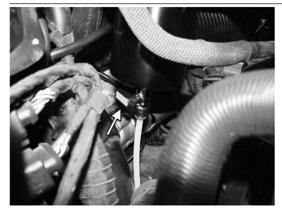
11) Confirm that the drain valve on the catch can is closed (parallel to the ground). The catch can can be drained by holding a cup under the drain valve and opening the valve.
