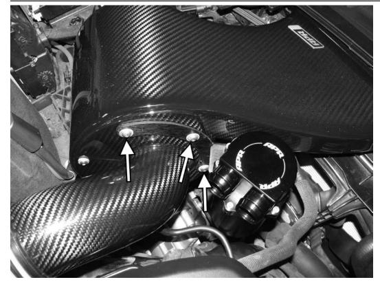
5) Tighten the three screws holding the catch can bracket to the intake. Make sure the seals begin to crush, but do not overtighten the screws.
