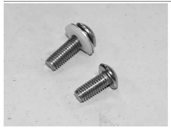
3) Transfer the seals and washers from the three airbox screws to the longer screws included with the catch can.
