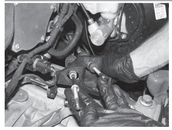
9) Slide the stock shifter cable bracket out of the car by sliding the bracket forward while pulling the cables through the holes in the bracket. Take note the location of each cable; the longer cable should be closest to the engine.
