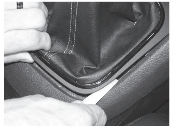
15) Once the back of the shifter surround trim is lifted up, use the trim tool to work on both sides of the shifter trim. Once removed, the shifter boot and surrounding trim can be lifted up above the shift knob. The boot does not need to be removed.
