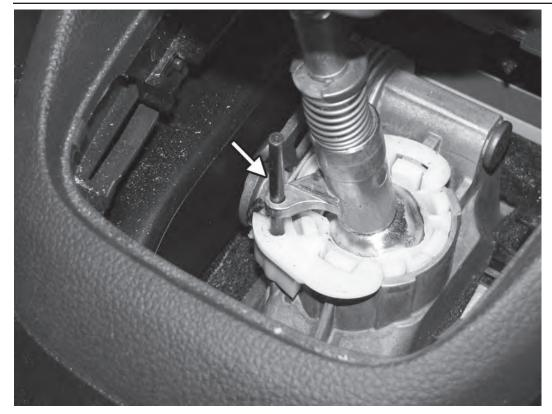
17) Pull the shifter back and to the left to align the hole in the shifter with the hole in the shift linkage. Use the supplied metal pin to lock the shifter in this location.
