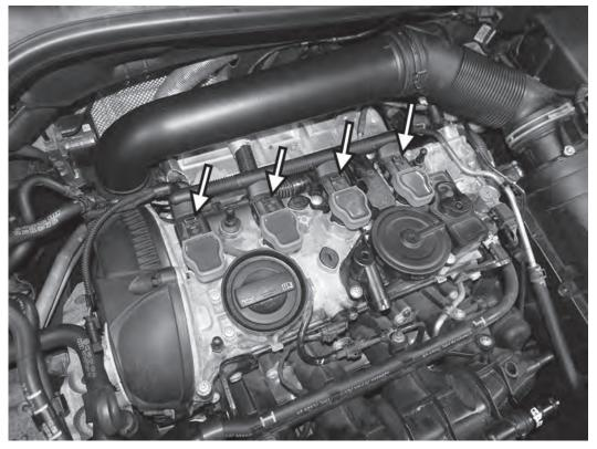
3) Disconnect the four electrical connectors to the ignition coilpacks, and lift the harness away from the coilpacks.
