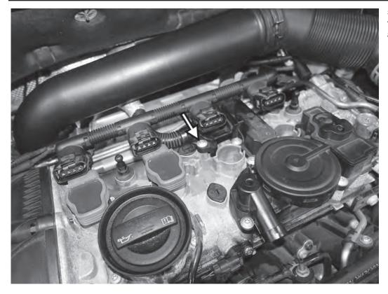
5) Remove the T30 screw from the vent line that connects to the oil separator on top of the valve cover.
