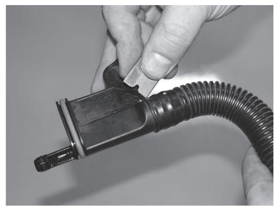
7) Remove the vent hose line from the plastic connection piece either by cutting off with a razor blade or by heating the connection with a heat gun and pulling it off.
