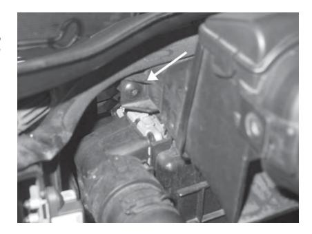
4) Disconnect MAF sensor and remove plastic compressor inlet hose.
