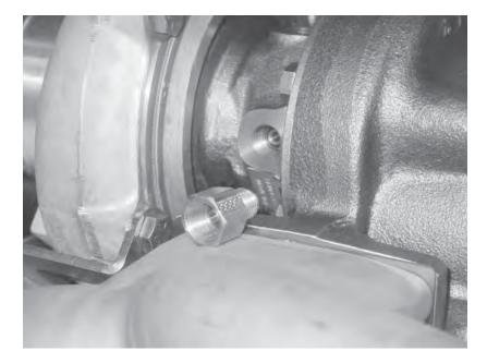
90) Install the oil feed line adaptor into the top of the turbocharger using a 5/8" socket.
