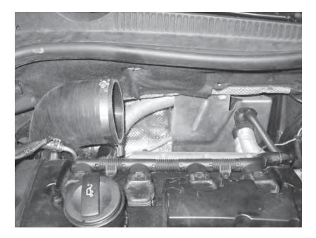
110) Remove the 5mm bolts and lockwashers and remove the APR MAF tube, leaving the compressor inlet hose in the car. It was necessary to install the MAF tube to get the correct orientation on the compressor inlet hose before tightening that hose in place.
