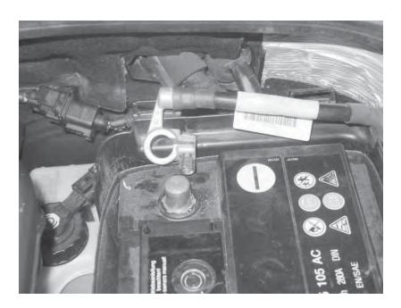
1) Support the car on jack stands or a lift. Open the hood and disconnect the 10mm negative battery terminal.
