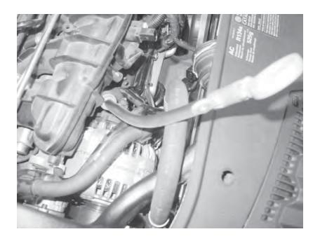
44) Connect the following electrical connectors on the intake manifold: plug under the intake manifold by the alternator, connector on drivers side of intake manifold and clip, EVAP purge valve, fuel pressure sensor, fuel pressure regulator, and fuel injector wiring harness.
