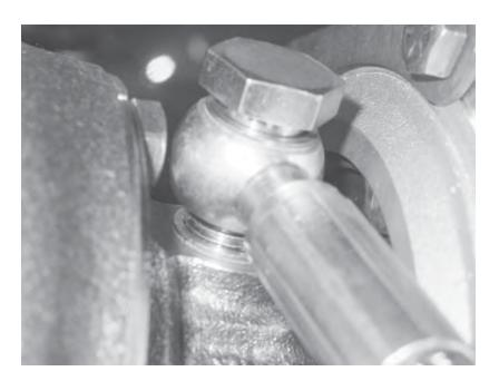
93) Install the other braided steel coolant line on the other side of the turbocharger. Again, install a crush washer on both sides of the banjo fitting, and tighten the 19mm banjo bolt.
