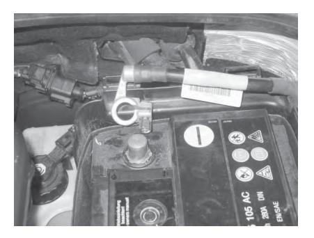
138) Reconnect negative battery terminal. Let the car sit for at least three minutes with the ignition key on and engine off. This is a good time to connect with a diagnostic tool and clear any error codes on the car.
