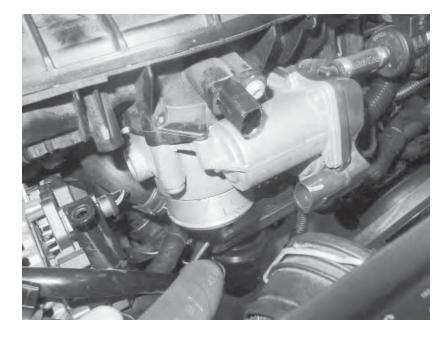
46) Set the throttle body back in place on the intake manifold and torque the T30 bolts to 89in-lbs in a crossing pattern.
