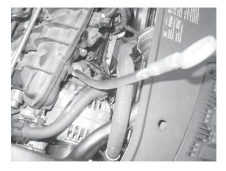
22) Remove the dipstick tube by pulling the assembly out and away from the block. Note the routing of the dipstick for later reinstallation.
