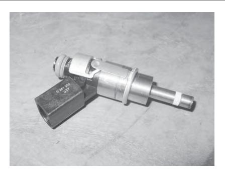
33) Preassemble the APR injectors with the new, supplied injector clips. The gaskets included in the installation kit are not needed with the new APR injectors.
