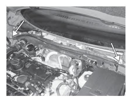
137) Reinstall engine ECU, noise resonance chamber, cowl panel, plastic cowl cover and windshield wipers.
