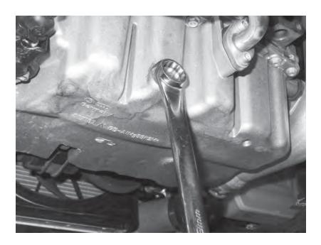
61) Drain the engine oil by removing the 18mm drain bolt from the bottom of the oil pan. It is advisable to change the oil filter on the car at this time as well.
