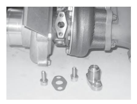
89) Install the gasket and oil drain flange to the bottom of the turbocharger using the supplied 6mm allen bolts.
