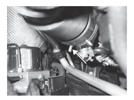
80) Remove the two 24mm plastic grommets that connect the stock airbox to the turbocharger heat shield. Also remove the four 10mm nuts on the back side of the heat shield, as seen from the back of the engine.
