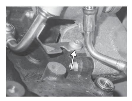
77) Loosen the 6mm allen bolt that connects to the oil line, but do not remove it.
