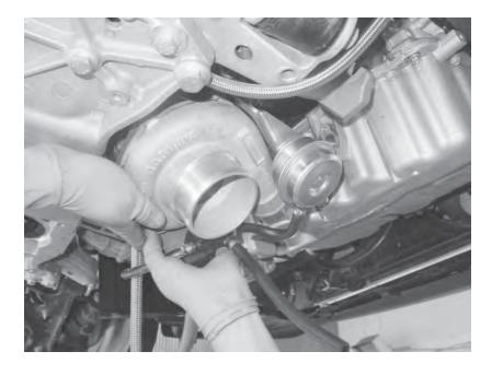
102) Lift the APR manifold/turbo assembly behind the engine as shown. Lift with the downturn end first as high as possible behind the engine, and then rotate the assembly into its correct orientation. Rest the manifold on the lower stock exhaust manifold brackets.
