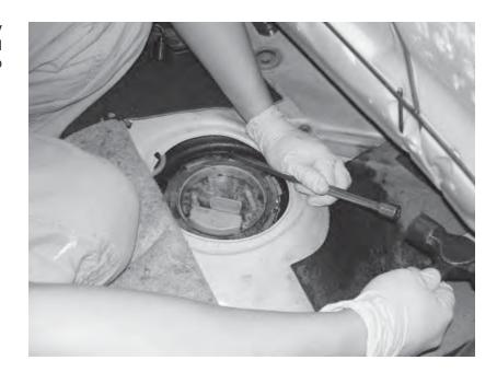
60) Lift the fuel pump housing out of the tank, being careful not to spill gas and not bending the fuel level float. Disassemble the housing and replace the fuel pump with the APR pump. Reinstall the fuel pump, reversing the order it was removed.
