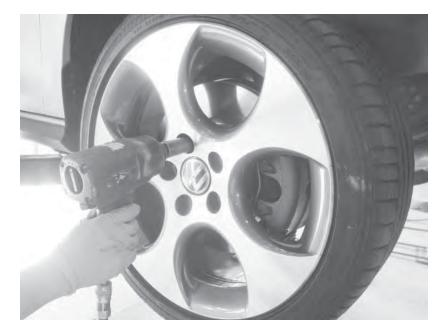
62) Remove the front passenger wheel and set aside.
