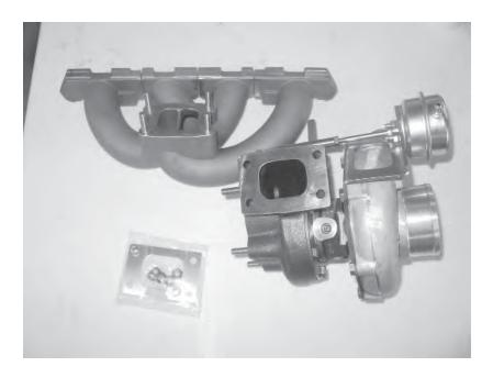
86) On a clean workbench, lay out the APR exhaust manifold, turbocharger, and turbo to manifold gasket set. Make sure all parts are clean and any debris is removed.
