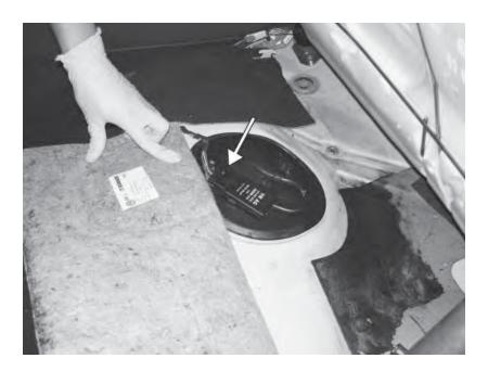
57) Flip up the bottom of the rear seat, but do not remove it. Under a carpet flap, you will see the access to the fuel pump. Disconnect the electrical connector on the plastic cover, and then pry the cover off carefully.
