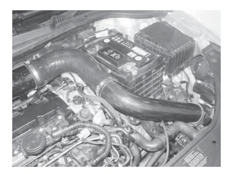
132) Remove the bolt nearest the inlet elbow and then install the air filter and clamp with attached bracket. Loosely install the bolt with the bracket, tighten the clamp on the filter, and then tighten the bolt.
