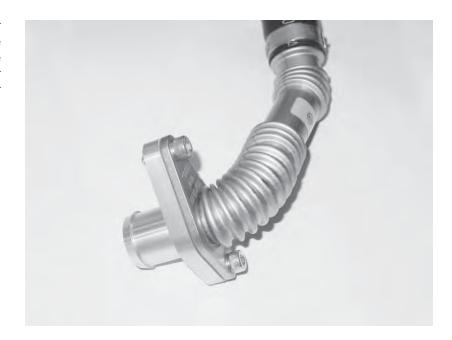
116) Install the supplied stepped bard fitting into the upper coolant line that was previously cut with a crimped hose clamp. Route the lower rubber coolant line off the turbocharger as shown, and connect to the upper coolant line from underneath. Install the other crimp clamp on the coolant line.
