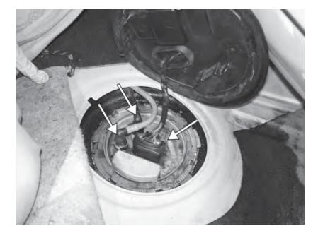
58) Disconnect the electrical connection from the pump housing. Also disconnect the two bundy connectors from the fuel fill and vent lines.
