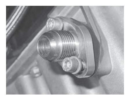
121) Install the oil drain line fitting onto the oil pan with the supplied gasket, 5mm allen bolts, and lockwashers. Install the oil drain line and tighten with a 1" wrench.
