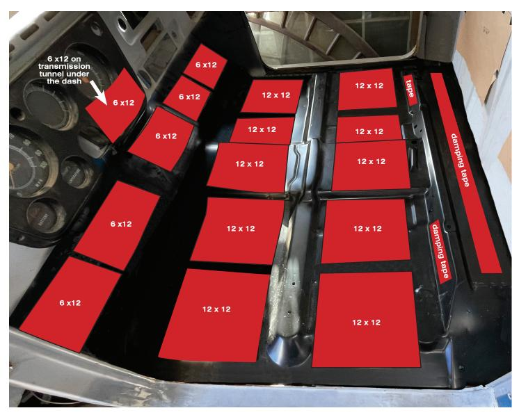
FIG. 2 Install damping matertial in these approximate locations. The perfect placement is not critical. But good adhesion is key. Make sure to press material in place with roller to ensure good adhesion. (View from driver side door)
