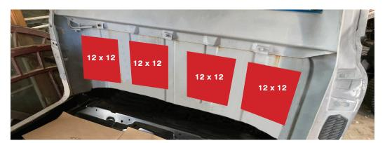
FIG. 3 Rear Bulkhead Install damping matertial in these approximate locations. The perfect placement is not critical. But good adhesion is key. Make sure to press material in place with roller to ensure good adhesion. (View from driver side door)
