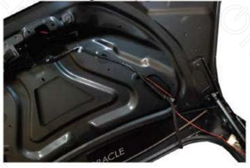
Unplug the taillight and take note of the wiring going into the Taillight Plug.
