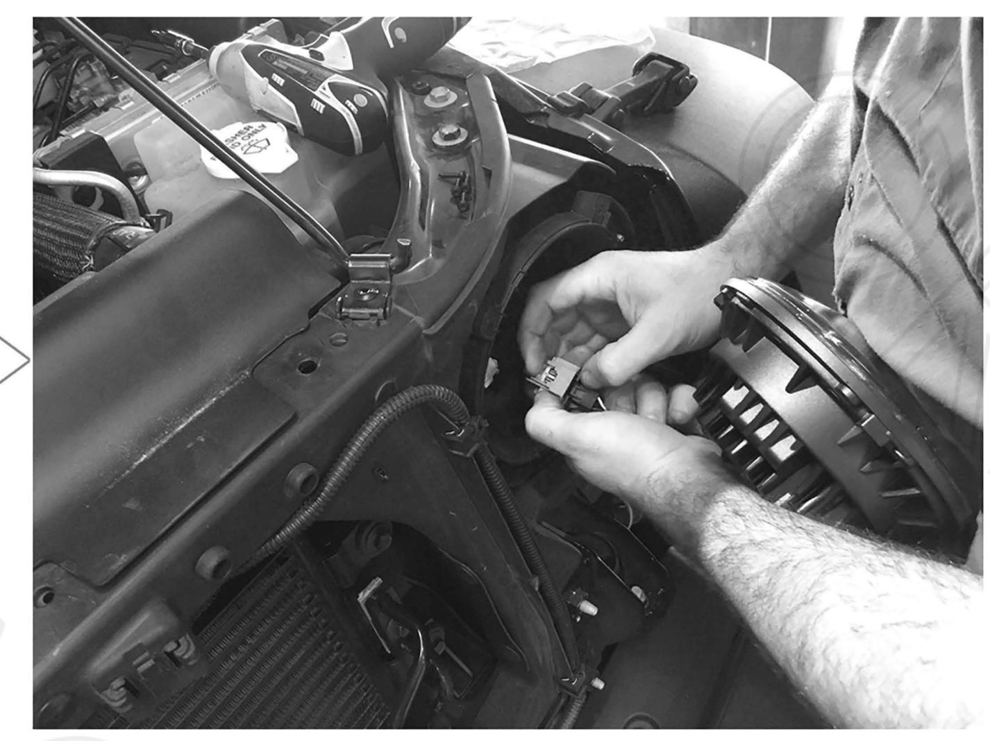
STEP 5: Slide Red Clip to Lock. If you can not squeeze together use a neddle nose pliers to slide the clip. Now Reverse Steps 1-3.
