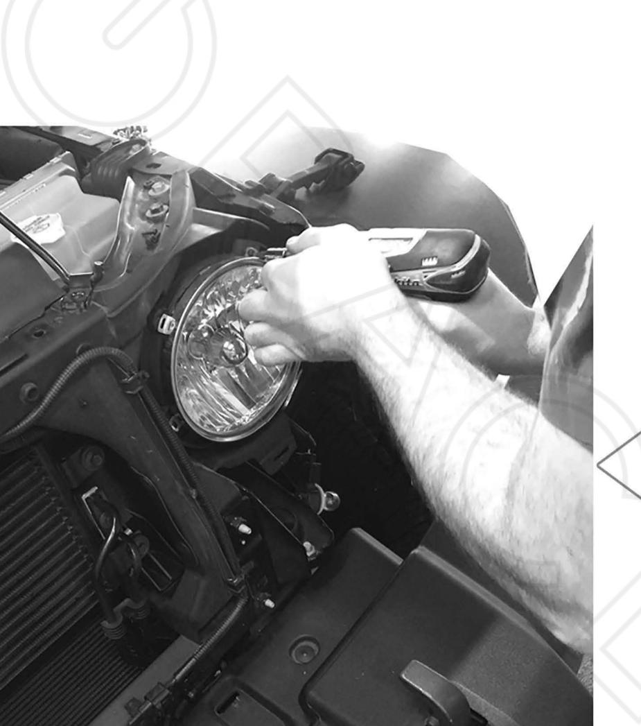
STEP 3: Remove the (4) T15 Torx Screws that hold the headlight trim ring bezel and lamp housing in place.
