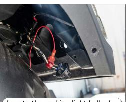
Locate the parking light bulb plug. T-Tap the red wire to the white with brown striped wire for power. Turn on park mode to test.
