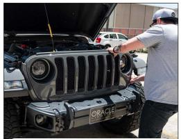
Use a panel tool or flathead to remove the retainer clips across the top. Firmly pull bottom of grill outward.
