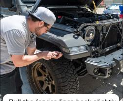
Pull the fender liner back slightly to access the park light harness. Remove the 3 outer fasteners.
