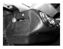
Drill (2) 9/32" holes for evaporator mounting.
