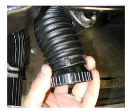
Locate drivers side louver. Remove ball louver and locate 2" dia. x 48" flex hose and attach to hose adapter using (1)  $\#10 \times 5/8$ " screw.
