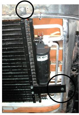
Slide condenser assembly between the Radiator and the radiator bulkhead.
