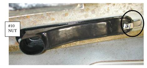
Locate in the unit box (2) Defrost Diffusers, and (2) #10 –32 nuts.
