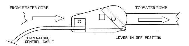
CAUTION: WATER VALVE MUST BE INSTALLED ON HEATER LINE ROUTED TO WATER PUMP.
