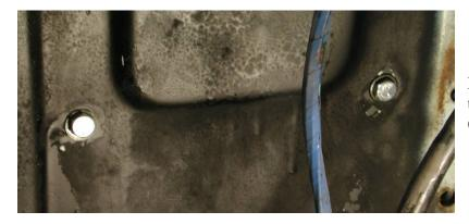
From engine side of the firewall attach unit using  $(2) \frac{1}{4}$  – 20 x 1" hex head screws and (2) flat washers.
