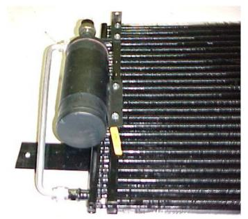
Attach drier, drier mounting bracket and liquid tube to condenser using (2) #10 screws, (2) #6 o-ring and a few drops of mineral oil on the connections.
