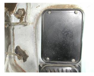
If truck is equipped with the deluxe heater. Remove the fresh inlet flange. Retain original hardware.
