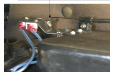
Attach (2) 3/16" spade terminals on blue wires to the micro switch located on top of the unit.
