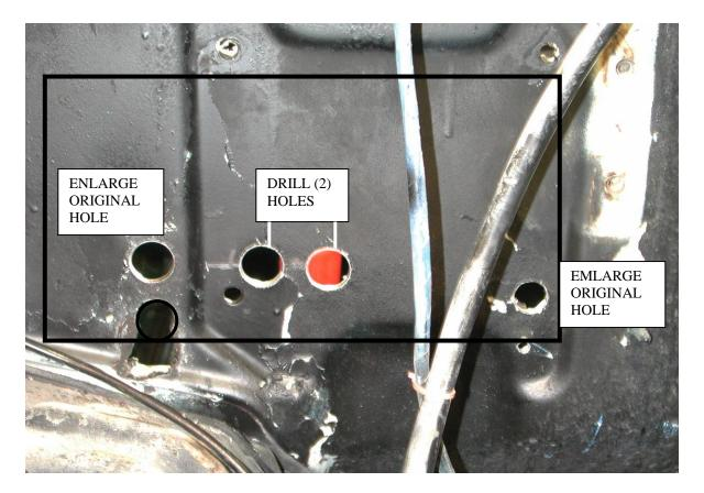
Enlarge original heater tube hole to 1" dia. Enlarge original heater mounting hole to 13/16" dia. Drill new heater tube holes to 7/8" dia.
