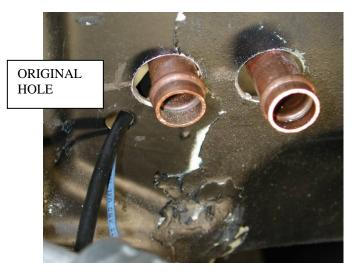
Locate Temperature Cable attached to the control head. Route this cable along firewall and out through original hole that supported the original heater.
