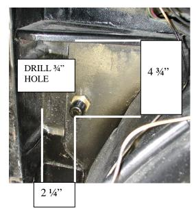
Located on the passenger side of the radiator bulkhead drill (1) hole  $\frac{3}{4}$ " dia.
