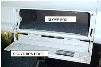
Remove the Glove box. Retain all original hardware. Discard the glove box housing.
