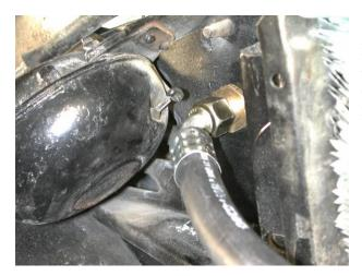
Route discharge hose from the bulkhead over to the compressor and attach end with service port to compressor using (1) #8 o-ring and a few drops of mineral oil. Tighten securely.
