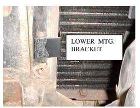
Locate in the condenser kit the lower right condenser mounting and (2) #10 x 3/8" hex head screws. Attach bracket to the condenser on third hole from the bottom.
