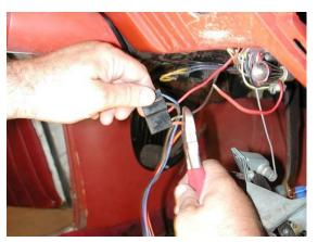
Locate original wire harness that was attached to the blower switch. Cut the connector off. Attach (1)  $\frac{1}{4}$ " male spade connector to the brown wire.
