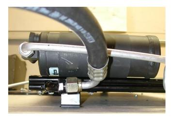
Carefully place Condenser Assembly through the Radiator Support as shown. Notice: on the next page slide the discharge hose through top grommet in the support. Route hose around battery towards the compressor.
