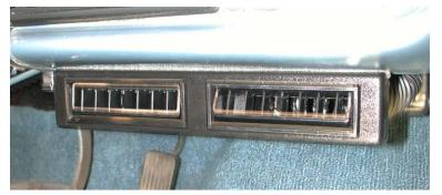
Locate Center Louver Bezel Assembly and (4) #8 x 3/8" pan head screws.
