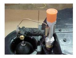
Install liquid line onto the Expansion valve (TXV) as shown. Use #6 o-ring and (2) drops of mineral oil on the o-ring and tighten securely.
