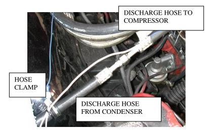
Fasten #8 hose to the fender well behind battery using hose clamp and (1) #10 tek screw..
