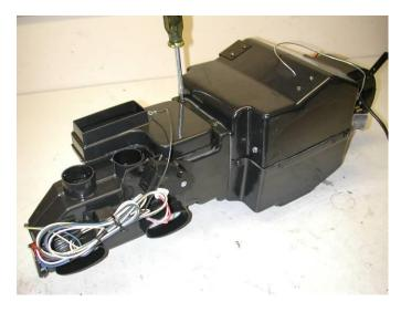
Locate the evaporator, Air Distribution Duct assembly and (4)  $\#10 \ge 5/8$ " pan head screws..
