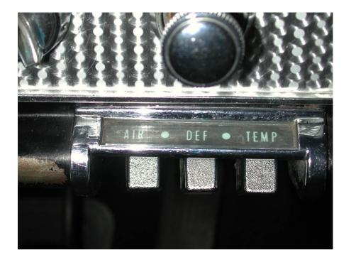
THE PICTURE YOU SEE ABOVE SHOWS THE CONTROLS IN THE FACE MODE. THIS MEANS THAT THE AIR WILL BE DISTRIBUTED THROUGH THE FACE OUTLETS. THIS ALSO HAS THE TEMPERATURE LEVER IN THE COLD POSITION. WITH THE CONTROLS IN THIS POSITION YOU WILL GET THE AIR THROUGH THE FACE OUTLETS WITH THE COMPRESSOR ON.
