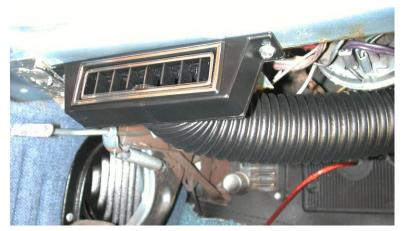
Route flex hose over to center distribution duct and attach to left outlet on side of the duct.
