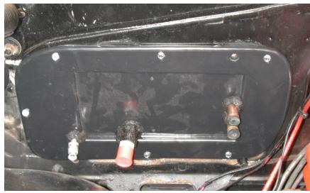
Locate the Firewall Block Off plate, and (6)  $\#10 \times \frac{3}{4}$ " hex head tek screws.
