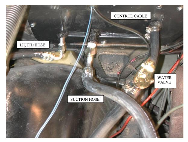
Locate the water valve and (3) worm gear clamps from the hardware sack kit.
