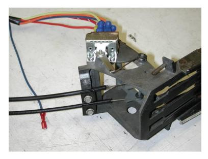
Attach (longest) temperature control cable using original hardware to bottom control arm and (1) 3/16" push nut. NOTE: Cable sleeve is 1/4" from the lever arm.
