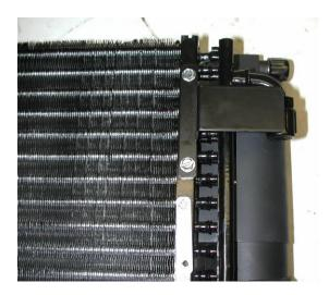
Locate the Condenser, (1) right condenser mounting brackets, and (2)  $\#10 \ge 3/8$ " hex head screws.
