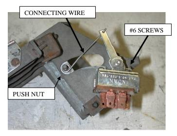
Locate the blower switch, (2)  $\#6 \times 3/8$ " pan head screws, (1) 3/16" push nut and the connecting wire from the control sack kit.
