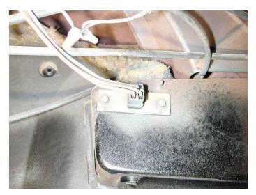
Locate behind the original control head on heater box, the resistor connector located on heater box..
