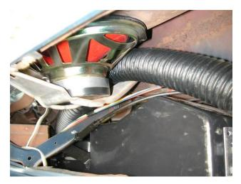
Route 2" dia x 40" flex hose from right outlet on top of the distribution duct across top of the evaporator and attach to the passenger louver assembly.
