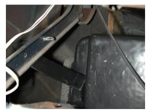
Locate in the hardware sack kit the evaporator support brace, (1)  $\#14 \times 3/4$ " tek screw.
