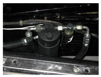
Locate the liquid hose, Hi / Low pressure switch assembly, wire harness and (3) #6 o-ring.
