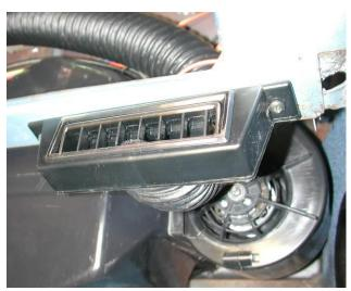
Locate in the hardware sack kit the remote louver assembly , and (2)  $\#10 \times \frac{3}{4}$ " hex head tek screws.
