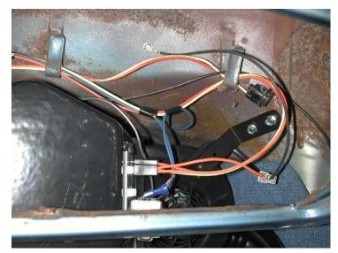
Route the main harness across front of unit to the resistor and blower motor. Route blue clutch wire over evaporator and out through the hole in the firewall above the unit. Secure ground from the blower motor using (1) #10 x  $\frac{3}{4}$  " hex head Tek screw. Also secure ground wire from electrical servo motor to the center brace using (1) #10 tek screw.
