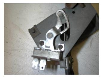
Locate the original control assembly. Remove and discard the original blower switch. Discard all original hardware.
