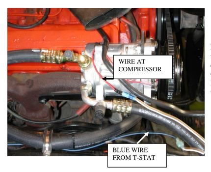
Route (1) of the white wires along with the #8 refrigerant hose. Attach to the compressor clutch. Other white wire attaches to Blue Clutch wire from the thermostat.
