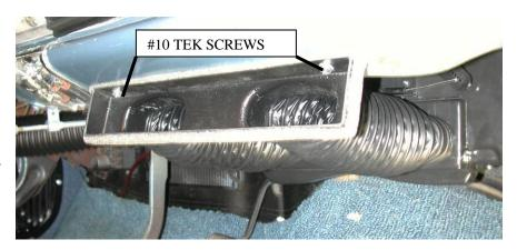
Attach 6" flex hose between center hose adapter and the distribution duct hose adaptors.
