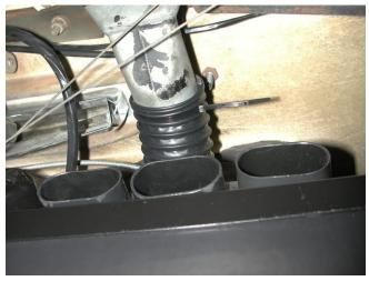
Flex hose from back of the unit needs to be routed over top and attached to the original defrost diffuser using (1) 6" tywrap.
