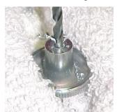
Carefully clamp the knob in a vice and drill a hole in the back using a  $\frac{1}{4}$ " diameter drill bit. Drill the hole  $\frac{7}{16}$ " deep.
