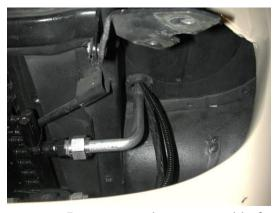
Locate the #8 discharge tube. Loosely attach to the condenser and insert through grommet hole as shown. This will locate the assembly from side to side.
