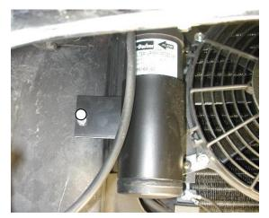
With condenser in place drill (2) holes on drivers and passengers side brackets through the bulkhead.
