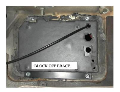
Insert the ½" screws through holes in the top and attach using the flange nuts.
