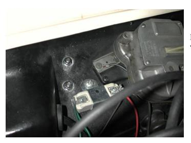
Passenger side bracket clamps to the body just above the unit. Loosely hang the unit.
