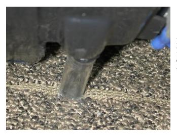
Locate clear drain tube from the hardware sack kit and attach it to drain fitting on the unit and out through the hole previously drilled.
