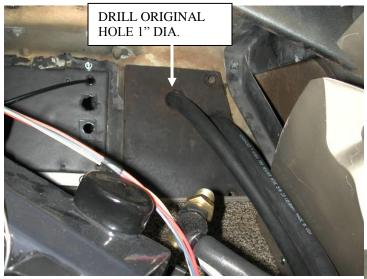
Locate on firewall original hole that the heater valve went through. Enlarge the hole using a 1" drill bit.
