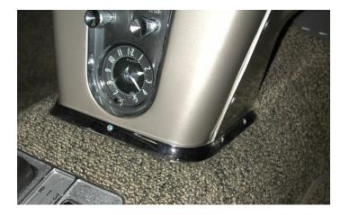
Remove trim ring at bottom of the console. Set aside and retain all original hardware.
