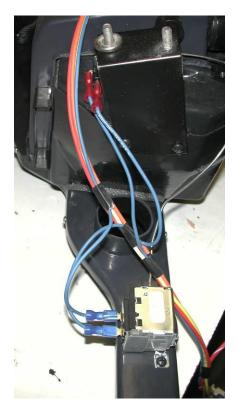
Locate in the control sack kit the wire harness. Attach harness to the resistor and ground wire at the motor. Route harness over top of the unit to the micro switch and thermostat. Connect the wiring per the wiring diagram below.
