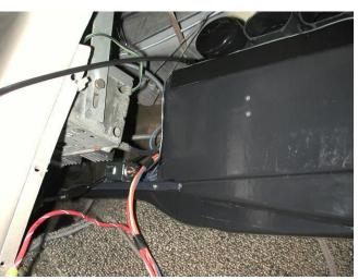
Insert studs through (2) holes next to windshield wiper. Attach using (2) 1/4"-20 flange nuts.
