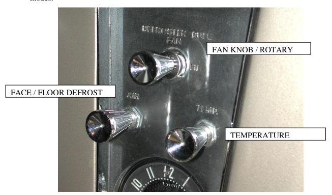
THE PICTURE YOU SEE ON THE FIRST PAGE SHOWS THE CONTROLS IN THE FACE MODE. THIS MEANS THAT THE AIR WILL BE DISTRIBUTED THROUGH THE FACE OUTLETS. THIS ALSO HAS THE TEMPERATURE KNOB IN THE COLD POSITION. WITH THE CONTROLS IN THIS POSITION YOU WILL GET THE AIR THROUGH THE FACE OUTLETS WITH THE COMPRESSOR ON.
