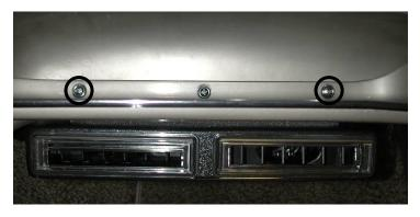
Reinstall passenger tray and install the passenger louver.
