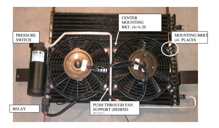
Attach fans and there mounting brackets to the condenser. Using hardware as shown on pg-19. Remove the bottom drier bracket screw and reinstall with bottom left fan mounting bracket.
