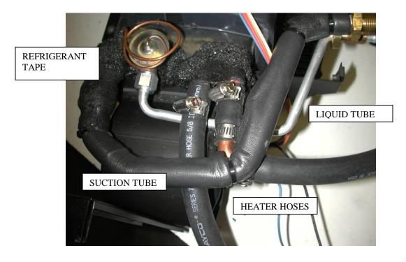
Locate in the hardware sack kit the Suction Tube, Liquid Tube, (1) piece of Heater hose 12" long, (1) piece 18", (2) worm gear clamps, (1) #6, and (1) #10 o-ring.
