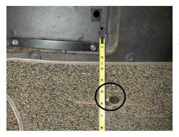
Locate and drill (1) 11/16" dia. hole 6" directly below bottom hole in the block off.
