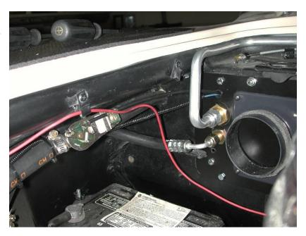
Locate Temperature Control Cable and attach it to the water valve as shown. Set cable so that the Temp knob is pushed all the way in and the water valve is in its fully closed position.
