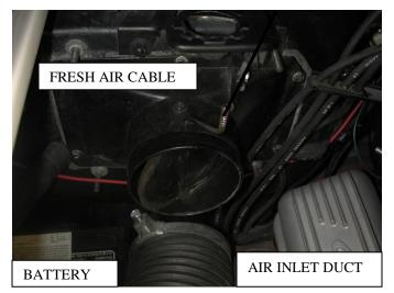
Disconnect battery ground cable.
