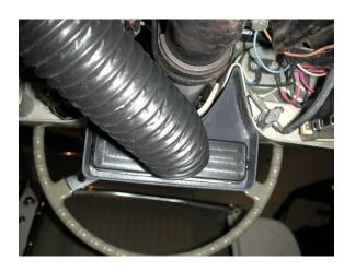
Reinstall trim bezel using original hardware.
