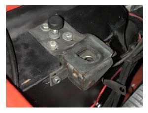
NOTE: 1958-59 Model vehicles remove the hood latch assembly.
