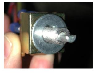
Locate in the control sack kit the large washer, small washer and the switch nut. The blower switch is on end of the wire harness.
