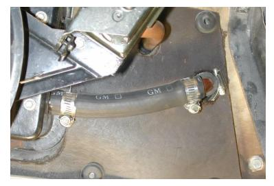
Locate beside heater assembly the return line to the engine.
