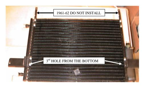
Install the condenser brackets as shown above.
