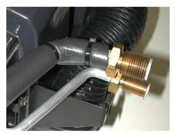
NOTE: The orientation of the refrigerant tubes.
