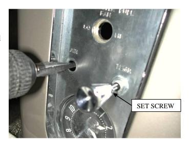
Install (1) of the control knobs that was modified to the shaft using the set screw.
