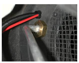
Locate the liquid line and (1) #6 o-ring.
