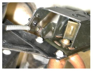
Located on engine side of firewall is the air inlet and door assembly. Remove (4) nuts around the outside of the housing.
