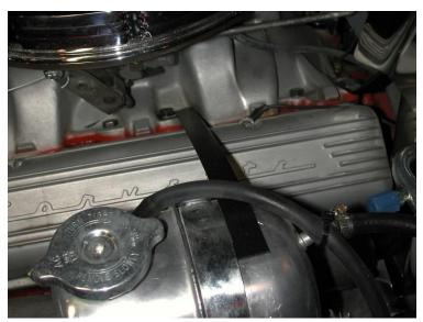
Locate upper support brace from the condenser kit. Remove the manifold bolt and attach the brace as shown.
