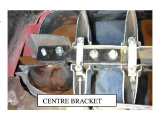
Remove cross brace from the grille on both sides and retain hardware.
