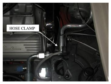
Locate suction hose and attach end with service port to rear of the compressor and back to the suction tube using (2) #10 o-rings and a few drops of mineral oil.
