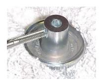
Locate the #8-32 thread tap and thread the hole.
