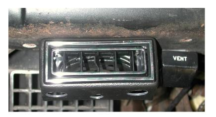
Locate 2" dia x 3ft flex hose from the unit box. Attach flex hose to the louver assembly using (2) #8 x 3/8" pan head screws. Route over steering column and attach to left outlet on the face / heat duct.
