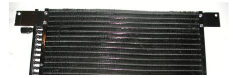
Remove light bezels and then the grill. Retain original hardware. Remove top radiator mounting bolts and retain. Loosen the lower mounting bolts.
