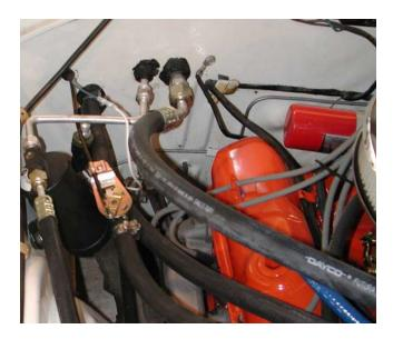
Locate the suction hose and (2) #10 o-rings. Attach end with the service port to compressor and the other end to the fitting at firewall. Use (1) #10 o-ring on each of the fittings and a few drops of mineral oil.
