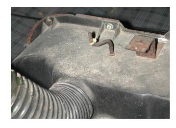
Also remove the defrost flex hose from drivers and passengers defrost outlet.
