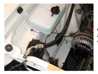
Other end routes along passenger inner fender and attaches to liquid tube from the condenser. Use (1) #6 o-ring and a few drops of mineral oil.
