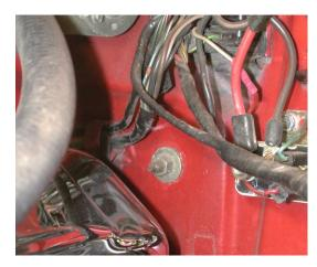
Locate on drivers side of firewall (1) nut that attaches the heater box.
