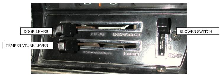
THE PICTURE YOU SEE ABOVE SHOWS THE CONTROLS IN THE HEAT MODE. THIS MEANS THAT THE AIR WILL BE DISTRIBUTED THROUGH THE HEAT OUTLETS. THIS ALSO HAS THE TEMPERATURE LEVER IN THE COLD POSITION. WITH THE CONTROLS IN THIS POSITION YOU WILL GET THE AIR THROUGH THE HEAT OUTLETS WITH THE COMPRESSOR OFF.
