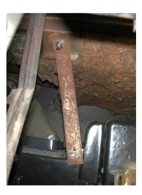
Locate original brace and (1) nut and (1)  $\#10 \times \frac{3}{4}$ " tek screw.
