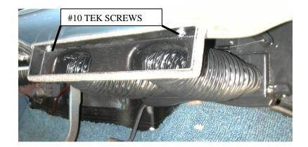
Attach 8" flex duct between center hose adapter and the distribution duct hose adapters.
