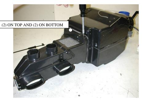
Locate the evaporator, Air Distribution Duct assembly and  $(4) \#10 \ge 5/8$ " pan head screws.
