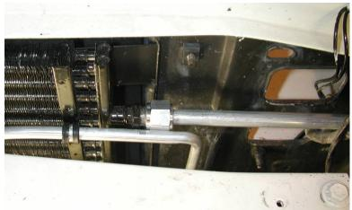
Locate (1) #8 hose clamp (1) #6 hose clamp, and (2) #10 tek screws.
