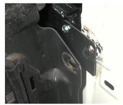
Top brackets line up to the upper radiator mounting bolts. Between radiator and the radiator support.
