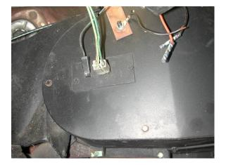
Disconnect Heat / Defrost cable from top of the heater box.
