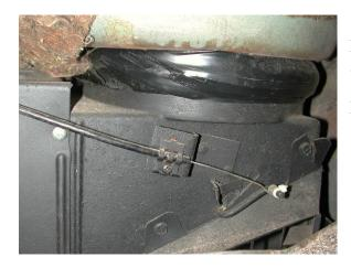
Remove push / pull assembly that was attached to the fresh air door.
