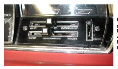
Locate Heater Controls below the gauges. Remove control knobs on the levers. Remove (2) screws on the control head face. Remove and retain the face and hardware.
