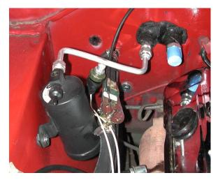
Locate the short Liquid Tube, (2) #6 o-rings, Receiver Drier, Hi/Low Pressure switch and (3) #10-32 x 1" screws and nuts.
