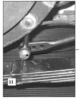
Attach end link to outer hole as shown before driving. DO NOT use inner holes until first driving vehicle with end link in outer position.
