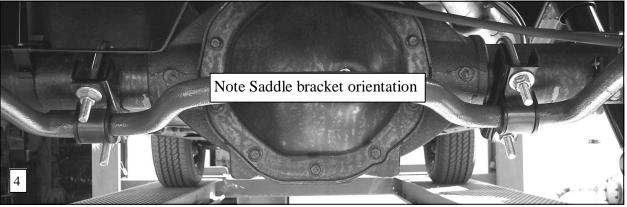
BEFORE INSTALLATION OF SWAY BAR ASSEMBLY, RELOCATE EMERGENCY BRAKE CABLE USING SUPPLIED BRACKET AND 5/16 BOLT AS SHOWN IN PHOTO (1).
