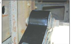
13) Before adjusting the coil spring to the correct tension, check to see that the eye bracket is in the center of the spring eye.
