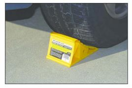
1) Before starting the installation make sure the vehicle is on a level surface, then place wheel chocks on both sides of the front wheels.
