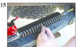
15) We have included with this kit two small discs, that are to be used as a gauge to adjust the tension setting of the variable rated tension coil springs. These can be adjusted to two different settings, depending on the vehicle requirement. For improved handling and 25% additional load carrying the correct adjustment between the coils is reached when the white disc (1mm thick) is used as a gauge and can just pass between the coils.
