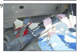
9) To lengthen the unit so the bolt spacer and nut can be located on the other side of the U bolt and under the bottom leaf spring. Start turning the coil spring with one hand and hold the threaded rod with the other.
