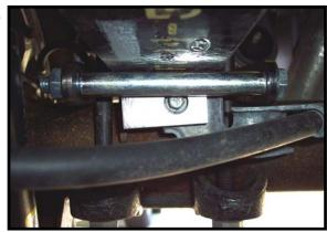
4) WITH THE BRACKET NOW IN PLACE, THE AXLE CONNECTING BRACKET CAN BE POSITIONED AS ILLUSTRATED IN INSTRUCTION 10 AND 11 AS PER THE FITTING INSTRUCTIONS.
