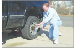
3) Position a floor jack of (the correct capacity for your vehicle) under the differential housing.
