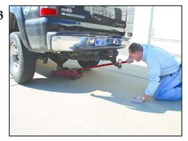
4) Next raise the rear of the vehicle with the jack sufficiently to place jack stands on both sides of the vehicle. As the vehicle has rear leaf springs, the ideal place to position the stands is under the front eye of the leaf springs, connected to the fixed shackles, as illustrated. With the floor jack still under the differential, next remove the rear wheels. With the lug nuts now loosened, this will make the removal a lot easier.
