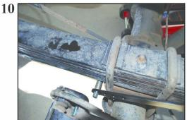
10) With the axle bracket now in positioned under the leaf springs, insert the connecting bolt and spacer as shown in the illustration.
