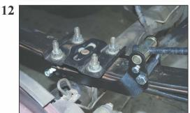
12) When fitting to some Ford vehicles where the U bolts are located around the axle and have a hold down plate on top of the leaf springs, the axle connecting bracket must be located the same way as in illustration  $(1\bullet)$  also with the bolt and spacer directly under the leaf springs (11).
