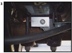
3) NEXT INSERT THE SCREW IN THE RECESSED HOLE IN OUR SMALL BRACKET AND THEN AS SHOWN IN ILLUSTRATION (3), SCREW IT BACK THROUGH THE HOLE IN THE PARKING BRAKE BRACKET AND THEN INTO THE HOLE IN THE LEAF SPRING PERCH.
