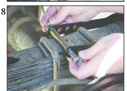
8) Next remove the nut, bolt and spacer. The bracket should now hang astride the leaf spring pack and U bolts.
