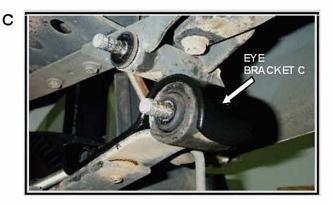
NOW POSITION THE EYE BRACKET (C) OVER THE EYE OF THE LEAF SPRING AND REPLACE THE SIDE OF THE SHACKLE THAT WAS REMOVED, AND SECURE THE TWO NUTS. REPEAT ON THE OTHER SIDE LEAF SPRING.
