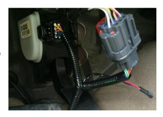
**Step 4:** Secure the PedalMAX unit using the (2) supplied cable ties. The device should not be hanging loosely or unsecured. Do not attach or mount to any moving assemblies such as the steering column.
