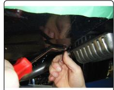
2. Lower exhaust by removing (6) rubber isolators.
