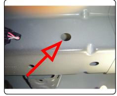
5. Remove nut from the post which is located on the inside of the frame rail, above the exhuast hanger, on the rearmost part of frame. Remove this nut from both sides.
