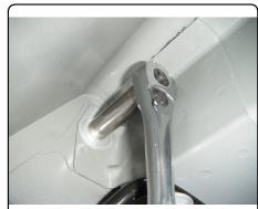
6. Raise hitch into position and attach to exsiting posts using the nuts that were removed in step 5.
