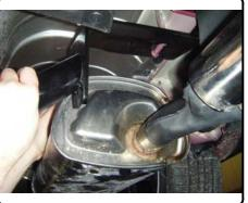
Loosely secure hitch with M10-1.25 x 25mm hex bolts and 3/8" conical toothed washers through existing weldnuts in outside of frame rails.
