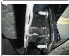
4. Lift the hitch into position over studs and secure with existing 12mm flange nuts.
