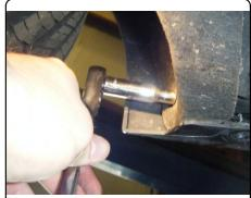
2. Remove (2) 12mm nuts from each bumper attachment. These will be re-used in STEP 4.
