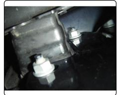
5. Fishwire 1/2" carriage bolts and SP-6 spacers into vehicle crossmember. (See FISHWIRE TECHNIQUE below) Note: If holes are not present, use mounting strap as a template to mark & drill 17/32" holes.
