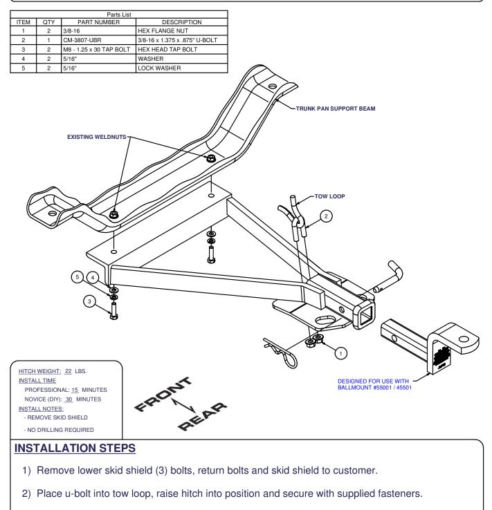
3) Torque all 3/8" fasteners to 45 lb-ft, and all M8 fasteners to 23 lb-ft.
