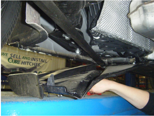
PLASTIC COVER REMOVAL (CONVERTIBLES ONLY)
