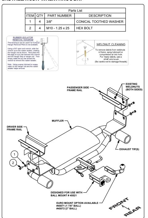
1. Lower exhaust by removing (2) rubber isolators from the exhaust side leaving the isolators attached to the vehicle. Exhaust will be supported by the rear axle. (see Rubber Isolator Removal Diagram)
