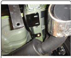
4. Torque all 12mm fasteners to 86 ft-lbs.
