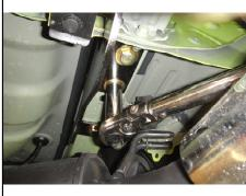
5. Trim underbody panel using trim diagram below for reference and reinstall panel and exhaust following Step 1 in reverse order.
