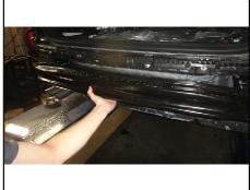
Place hitch between bumper beam and vehicle. Secure with supplied (3) M8 bolts and conical washers and (4) M8 bolts, lock washers, and washers. Torque all M8 bolts to 23 ft-lbs. Reinstall bumper cover following Steps 1-4 in reverse order. <u>NOTE:</u> For Golf Sportwagen vehicles with 4MOTION see TRIM DIAGRAM on Page 2.
