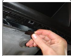
4. Remove bumper cover by gently pulling the bumper cover from the location of the nuts for the bolts removed from the wheel well and the bottom of the wheel well on both sides. Gently pull the bumper cover from the wheel well area toward the rear of the vehicle on both sides. Continue pulling straight back using a flat screwdriver to detach clips retaining the bumper cover as needed. Carefully remove the lower panel from the rest of the bumper cover.
