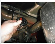
2. Temporarily remove driver side underbody panel by removing (3) clips using a flat head screwdriver and (4) nuts using a 10mm socket.
