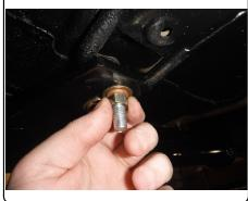
5. Torque M10 hardware to 48 lb-ft (if applicable), M8 hardware to 23 lb-ft (if applicable) and 3/8" hardware to 26 lb-ft.
