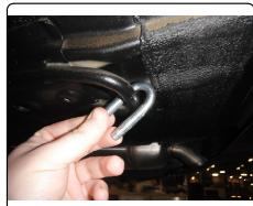
4. Raise hitch into position and slide u-bolt through holes in hitch. U.S.A. Built Models: Secure hitch to vehicle using supplied M10 bolts and 7/16" conical toothed washers. Korean Built Models: Secure hitch to vehicle using supplied M8 bolts and 3/8" conical toothed washers. Fasten to vehicle into locations where bolts were removed in step 3. (See CONICAL TOOTHED WASHER ORIENTATION DIAGRAM)
