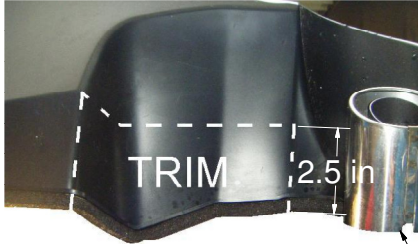
TRIM DIAGRAM FOR 2011 MODELS (PASSENGER SIDE SHOWN - TRIM BOTH SIDES)
