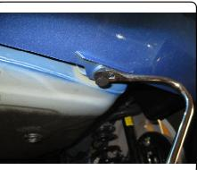
2. Remove one (1) M8 bolt on passenger side frame rail using a 13mm socket. Pull plastic away from frame rail as shown in photo below.
