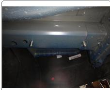
2. Raise hitch into position and secure with (4) 7/16" flange nuts, (2) each side. Torque 7/16" hardware to 70 ft-lbs.
