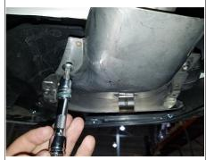
2. To lower exhaust, remove (2) bolts using an E12 socket from the exhaust bracket on each side. Locate and remove (2) rubber isolators from the exhaust towards the front of the vehicle.
