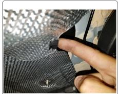
4. On the heat shields mark out a 4" x 8" section using masking tape and trim out using aviation shears. Reinstall heat shields using hardware from Step 3.
