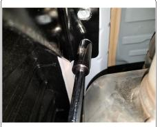
9. Torque all 7/16" hardware to 59 ft-lbs. Reinstall exhaust tips and raise exhaust following Step 1-2 in reverse order.
