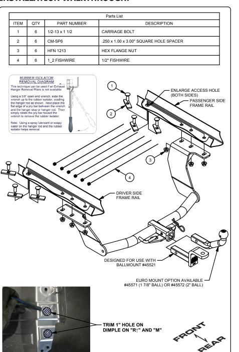
1) Lower exhaust by removing (3) rear rubber isolators. See RUBBER ISOLATOR REMOVAL DIAGRAM. If needed to access outside hangers remove plastic underbody panel by removing (7) plastic fasteners. NOTE: Support the exhaust as required.
