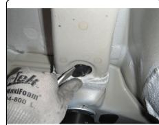
4) Fishwire the 1/2" hardware through the access hole into position on both sides, as shown below. Reinstall heat shield with (3) of the fasteners, without using the fastener between the hitch mounting holes.
