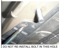
5) Raise hitch into position and loosely install1/2" hex flange nuts. **Note:** The heat shield will be between the hitch and vehicle frame rails.
