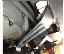
2. Raise hitch into position and install supplied fasteners as shown. Torque all 3/8" fasteners to 45 lb-ft and all 5/8" fasteners to 210 lb feet. Re-install remaining bumper fascia tabs to original positions.
