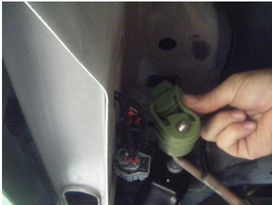
EXHAUST HANGER REMOVAL
