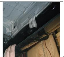
2. Remove (2) M8 fasteners for the driver side exhaust bracket, and (2) M8 fasteners for the muffler hangers using a 13mm socket. Support the muffler to prevent damage to the exhaust.
