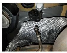
2. At the bottom of the wheel well, locate and remove (6) push pins, (3) on each side using a pry tool. Pull back part of wheel well to reveal (4) push pins, (2) on each side and remove using a pry tool.
