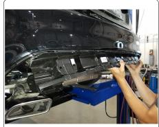
6. Place bumper beam onto hitch aligning the studs with the holes on the hitch. Raise hitch into position with the bumper beam, tucking them underneath the bumper fascia and then twisting bumper beam to reinstall. Loosely fasten using nuts removed from Step 5.
