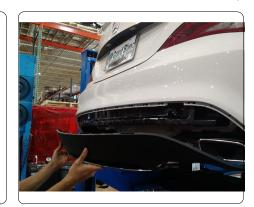
5. Locate the bumper beam connection points and remove (8) nuts, (4) from each side using a 16mm socket. Remove bumper beam by pulling bumper towards rear of car while twisting the bumper beam up towards the top of the vehicle. Set aside for later reinstallation. **NOTE:** Use silicone sealant around openings of the frame rail on each side as shown in FIGURE 1.
