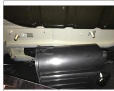
8. On driver side frame rail locate and remove (1) nut using 10mm socket.
