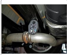
4. Locate and remove (2) plastic nuts with a 10mm socket. Remove heat shield and mark out a 5" x 13" section with masking tape. Use aviation shears to trim marked area. Reinstall with (1) nut using a 10mm socket.
