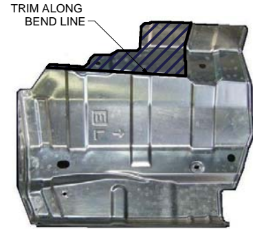
HEAT SHIELD TRIM DIAGRAM
