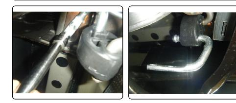
4) Raise the hitch into position and install (3) 10mm bolts and conical toothed washers per side into the existing weldnuts in the frame. If the vehicle is all wheel drive then reinstall the sway bar brackets using CM-SP50 spacer blocks and the existing nuts on the lower mounts.
