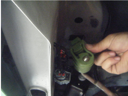
EXHAUST HANGER REMOVAL
