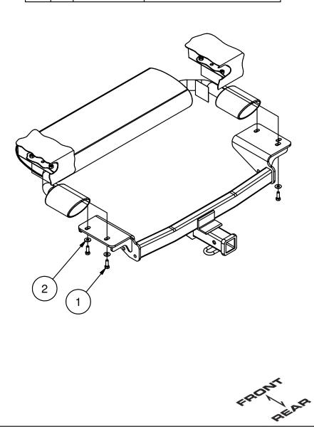
1. Locate weldnuts in frame rails (see Weldnut Cleaning Diagram).
