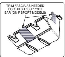
16. Using masking tape, layout the area to be trimmed, as shown. Use a rotary tool (or aviation shears) to trim the fascia.
