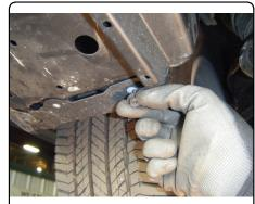
6. Fastener (9) is hidden behind wheel well trim. Pull back wheel well trim and remove plunger style fastener.
