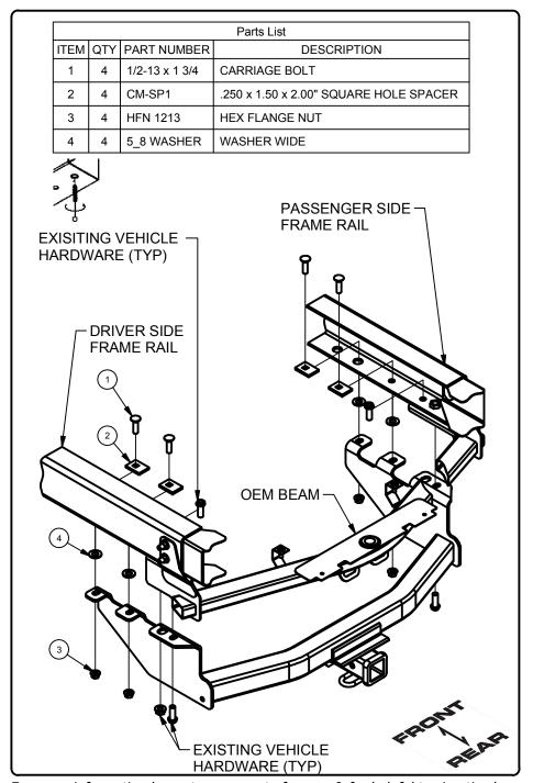
NOTE: For ease of install temporarily lower spare tire, See owners manual.
