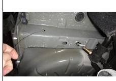
Slide the hitch in from the rear passenger side of the vehicle over the exhaust and into position. <u>Note</u>: Feed the fishwires through the mounting holes while raising the hitch.
