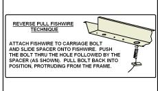
5. Remove the fishwires from the carriage bolts in the bottom of the frame rails and loosely secure the hitch with 7/16" flange nuts. Pull the fishwires through the side mounting holes and loosely secure them with 7/16" flange nuts. Re-attach the muffler brackets to the bottom of the hitch into the original mounting holes using the provided M8-1.25 hex bolts and 5/16" washers.
