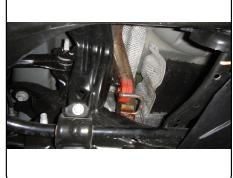
Remove the (1) fastener securing the heat shield to the bottom of the driver side frame rail. Trim the portion of the heat shield covering the mounting areas of the driver and passenger side frame rails, see trim diagram. After trimming re-attach the heat shield to the bottom of the driver side.
